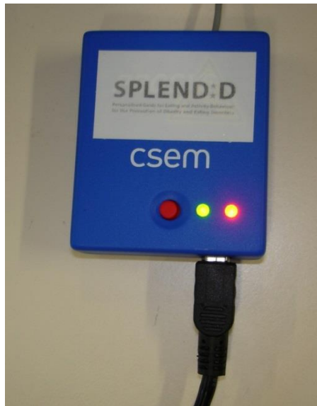
Figure 17: Recharging of the data logger
